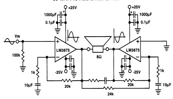
This audio power amp will deliver 80 W of audio into an  $8-\Omega$  load. The LM3875 IC devices should be suitably heatsinked. Note that the amplifier is a bridged circuit, with both speaker leads "hot."
